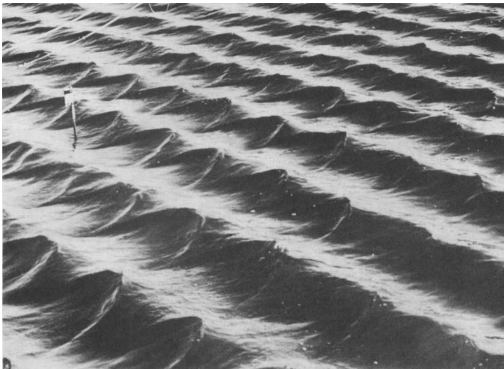
FIGURE 10. Three-dimensional symmetric waves of L_2 configuration observed in the wide wave basin; f_0 = 1.2 Hz, a_0 k_0 = 0.33 .
